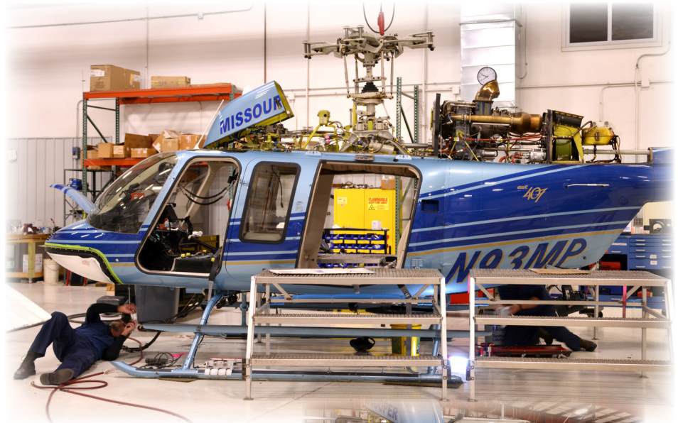
Aircraft Maint. Sprv. Doug Lauf (r) removed a fuel pump while Aircraft Maint. Spec. Kevin Schaperclaus detaches the current chin bubble from the Bell 407 helicopter.
