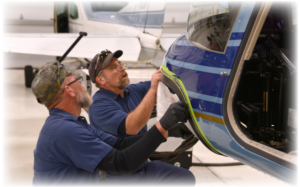
Aircraft Maint. Sprv. Doug Lauf and Aircraft Maint. Spec. Kevin Schaperclaus install a new chin bubble on the Bell 407 helicopter.
