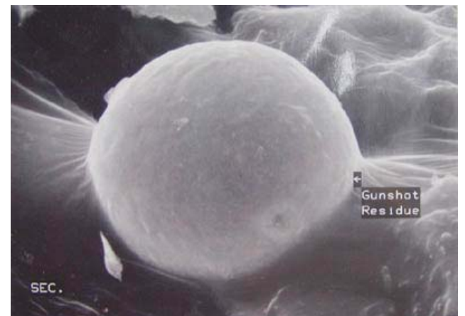
The round, white object is an actual GSR particle that has been magnified approximately 10,000X by a scanning electron microscope.
