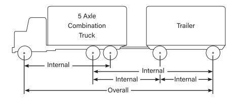
10-foot wheelbase from axle four to five allows 40,000 pounds. These two examples for gross weight purposes would be determined by the internal wheelbase from axle two to five. Take the total wheelbase measurement from axle two to five. This would be the critical measurement as 34 feet from axle two to five applied to the four axle column would allow a gross weight of 64,500 pounds.
